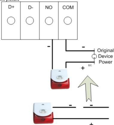
2. DO need a siren/buzzer. For example we are use a siren that use DC12V.
